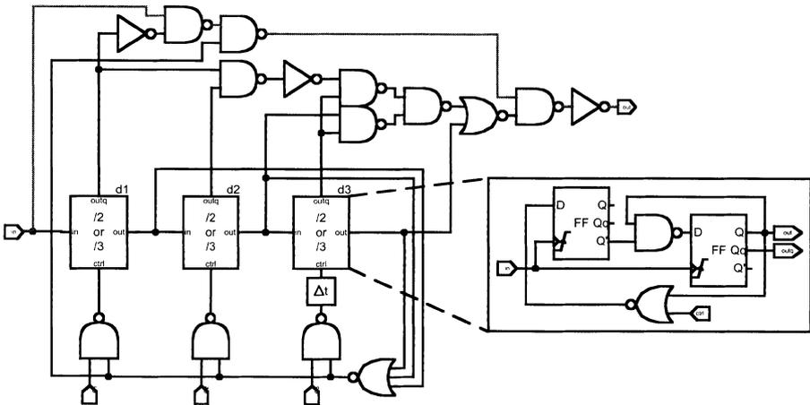
Fig.11. Improved PSRR design of a prescaler.
