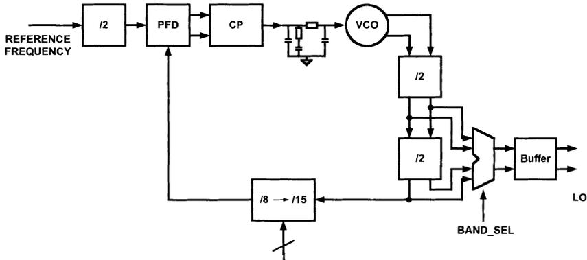
Fig.8. Architecture of the synthesizer.
