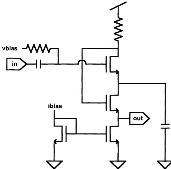
*Fig.3. LNA topology that re-uses the current.*
