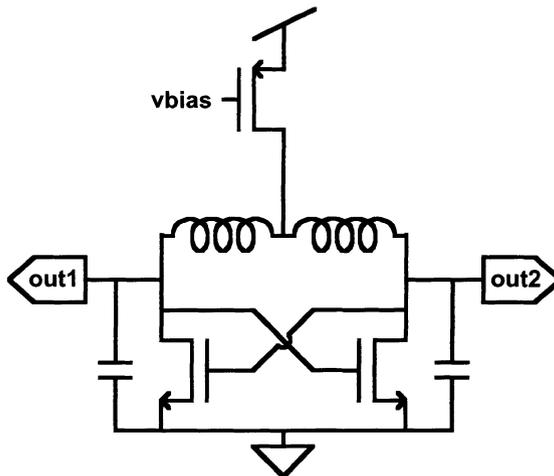
*Fig.2. Basic topology of a differential LC oscillator.*
