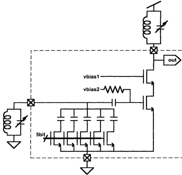
*Fig.6. Schematic of the LNA.*
