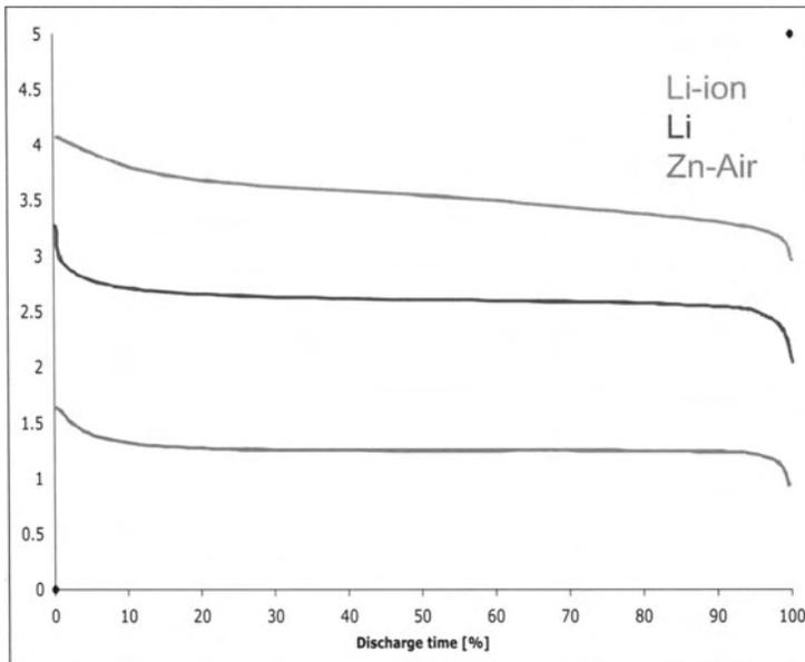
Fig. 1. Example discharge curves of commonly used battery types.
