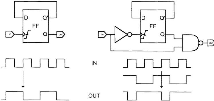
Fig.10. Improved PSRR design of a divide-by-2 block.
