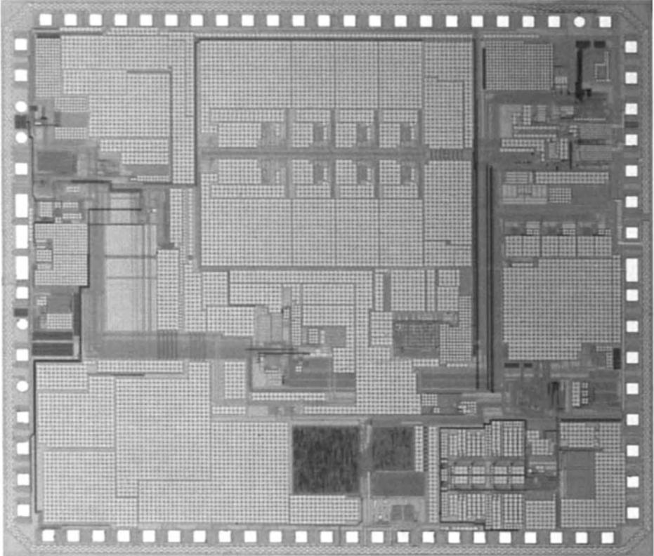
*Fig.12. Microphotograph of the FM receiver.*
