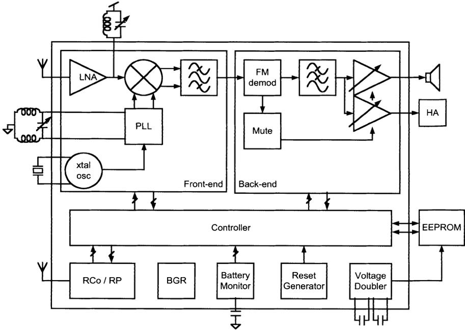
*Fig.4. Architecture of the low voltage FM receiver.*
