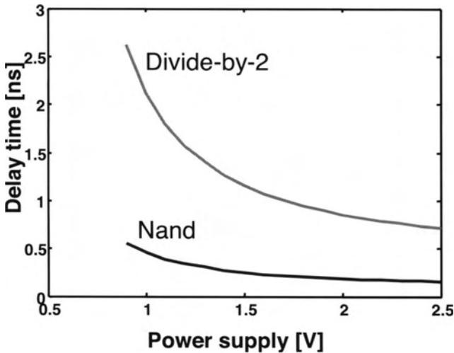
Fig.9. Delay time of digital cells i.f.o. the power supply.
