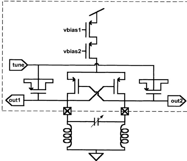
Fig.7. Schematic of the LC VCO.
