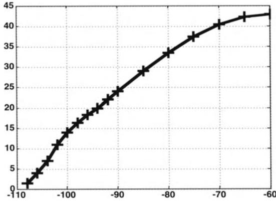
*Fig.13. SNR in function of the input signal power.*
