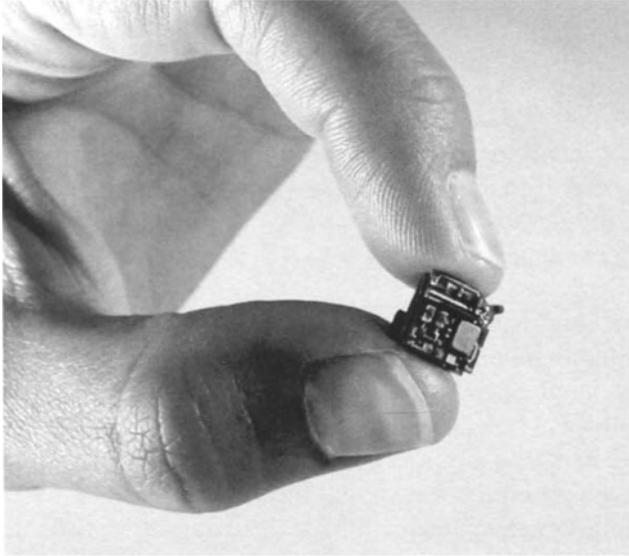
*Fig.5. The complete miniature FM receiver module.*
